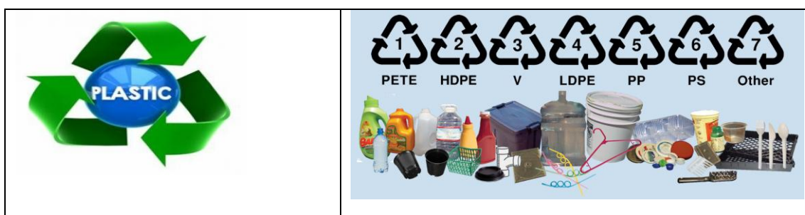
Figure 16. Plastic materials are categorized in numbers 1-7, the number represents the resin identification code associated with the type of plastic used and indicates the item's ability to be recycled
